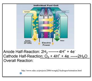
Anode Half-Reaction:  $2H_2 \longrightarrow 4H^+ + 4e^-$ Cathode Half-Reaction:  $0_2 + 4H^+ + 4e^-$ Cathode Half-Reaction:  $0_2 + 4H^+ + 4e^-$ Overall Reaction:  $0_2 + 2H_2 = 0$ http://www.odec.ca/projects/2006/wong6j2/hydrogenAnimation.html
